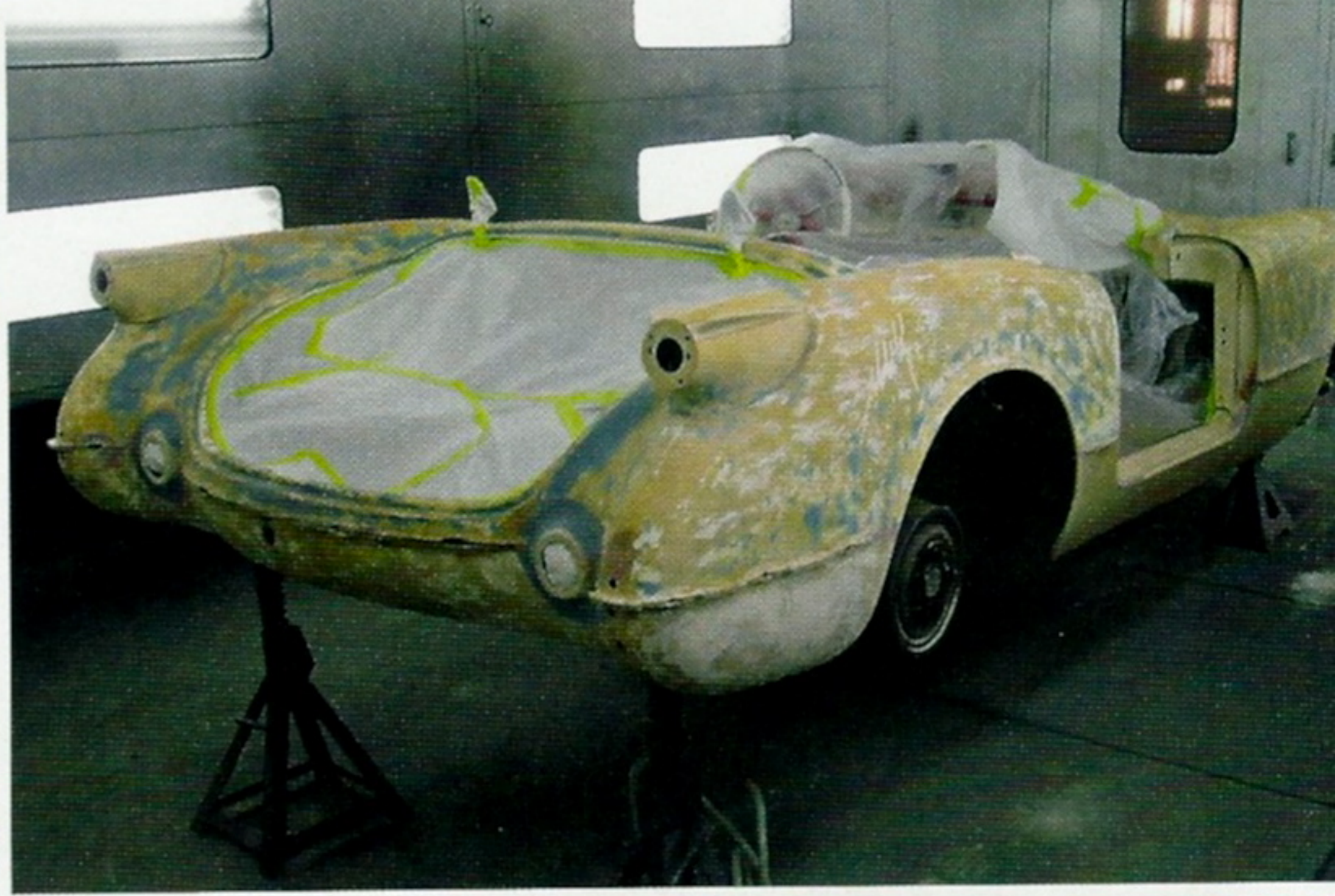
Above, left: Separating the body from the chassis was the first major step of the restoration; decrepit fiberglass needed lots of attention before being painted.
