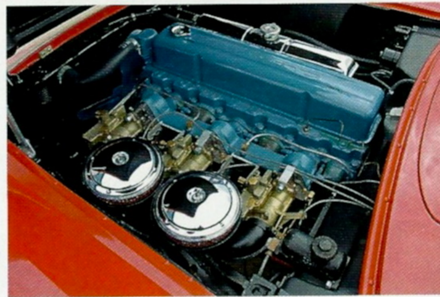
Right: Original 235-cid Blue Flame inline-6 looks like new, and puts out 138 horsepower at the rear wheels.
