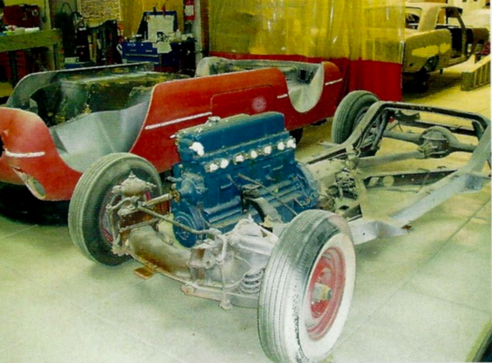
Above, left: Separating the body from the chassis was the first major step of the restoration; decrepit fiberglass needed lots of attention before being painted.
